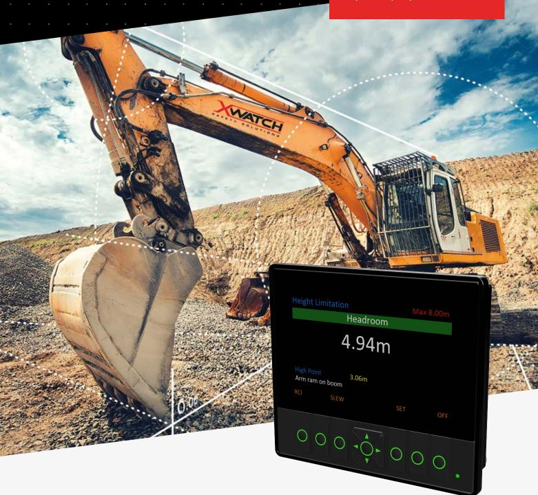
The XW4 can be configured to work on a variety of articulated hydraulic plant. Height and slew limitation is controlled using proportional soft-stop hydraulic valves providing accurate and repeatable performance without detriment to the machine.
